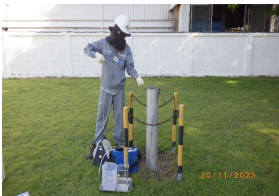
monitoring well (Up gradient) (GPS 47P 673047, 1576406)
